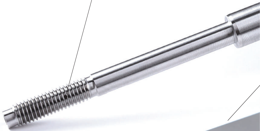
16ER 100ISO AP220U threading insert, used in threading operation of turbine shaft.
